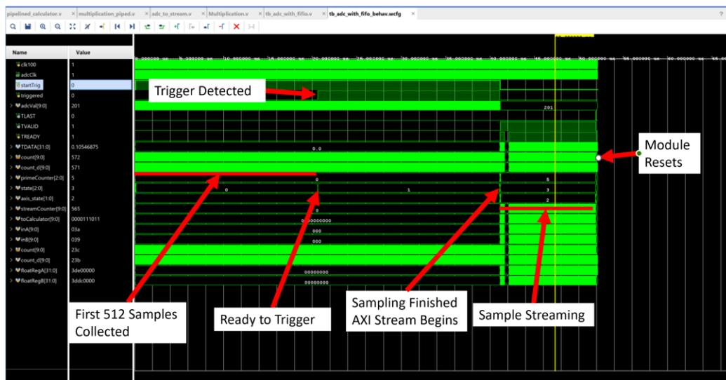
Figure 34: Test Bench of module
