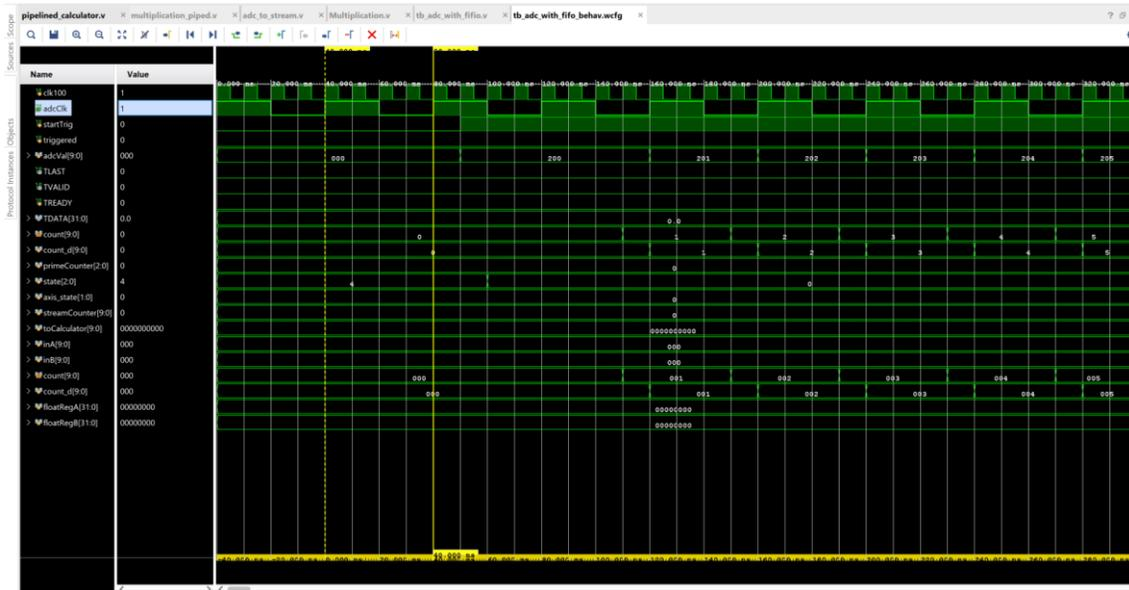
Figure 35: An example of running the ADC clock at a lower frequency (25MHz)
