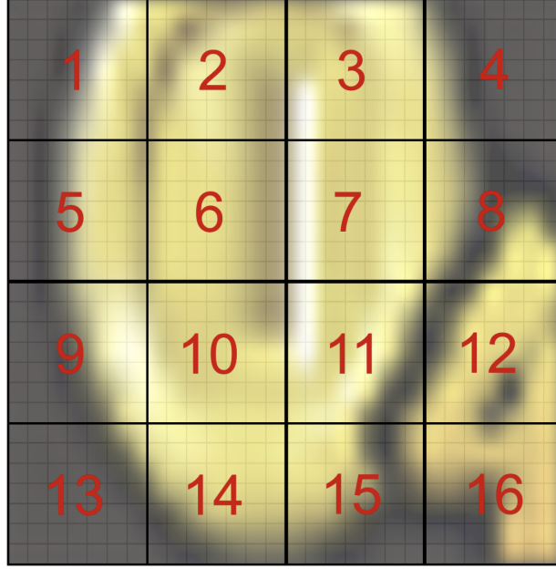
Figure 16: The image from the coin tile test broken into 16 7 x 7 pixel sections as is done in the bilinear interpolation block.
