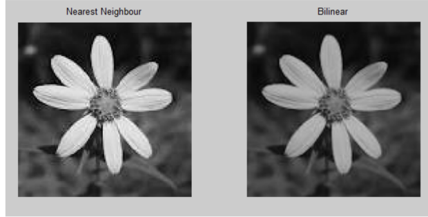
Figure 6: A comparison of nearest neighbor and bilinear interpolation on an upscaled picture of a flower [5].
